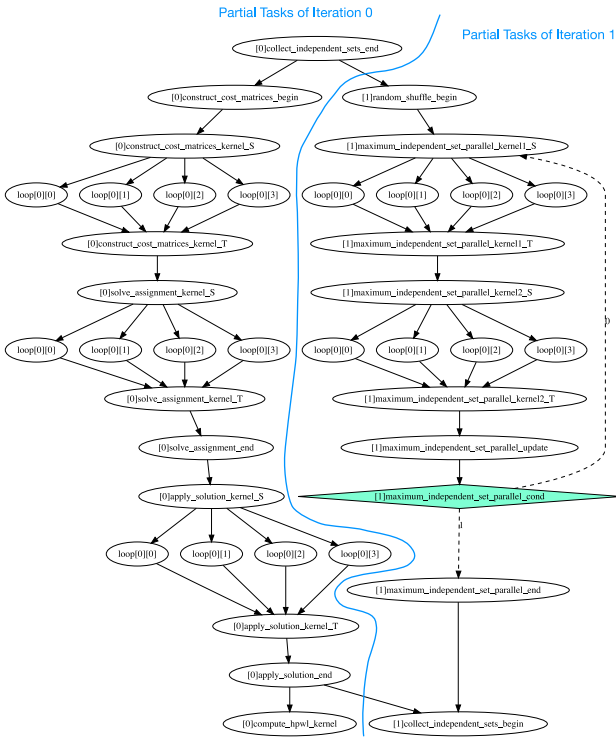
Fig. 14. Partial task graph for the detailed placement algorithm in Fig. 13. Steps of two consecutive iterations overlap in the task graph.
