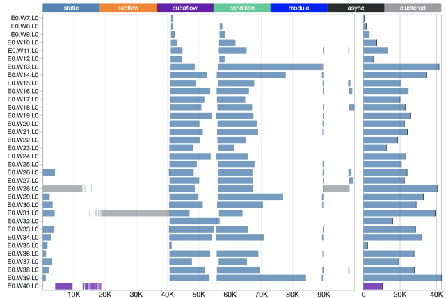
Fig. 12: Visualization result of a VLSI placement workload (partial taskflow graph shown in Figure 2) that incorporates 1.7M CPU-GPU dependent tasks [15]. The rendering time is about 981 ms for each selected range of tasks.
