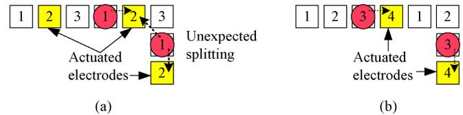
Fig. 19. Synchronized droplet movements require at least four control pins to prevent the fluidic error. (a) Three pins for droplet routing. (b) Four pins for droplet routing.
