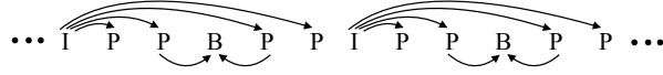
Fig. 1. A sample dependency diagram in a video encoding application of an x.264 standard. Edges denote the dependencies between two frames. I denotes frames, P denotes predicted, B denotes bi-directional frames.
